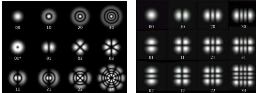
Depending on the geometry of the cavity - The left figure corresponds to circular cavities, and the right ones correspond to the square cavities.
